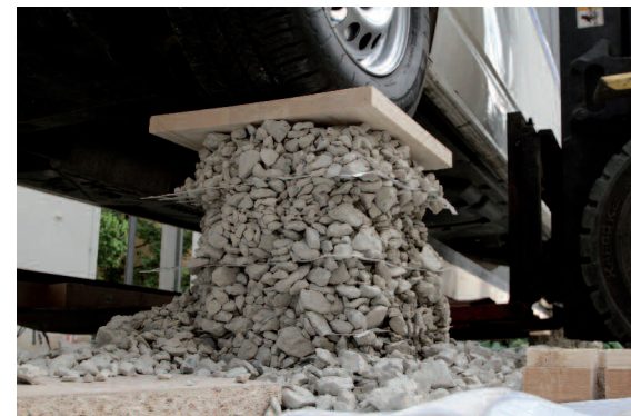
Figure 2 Demonstration of the interlocking effect under a 2.2t van
